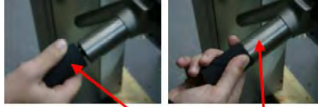
2. Make sure that the plastic part of the mini-arm is fixed to the steel part.
