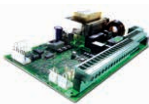
JE275 bollard control board controls 1 J355 M30-P1 bollard
