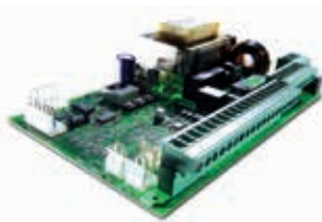
JE275 bollard control board controls up to 3 bollards type J275 HA
