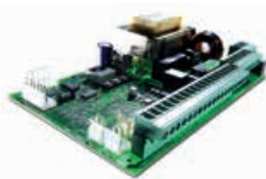
JE275 bollard control board controls up to 4 bollards, type J200 HA
